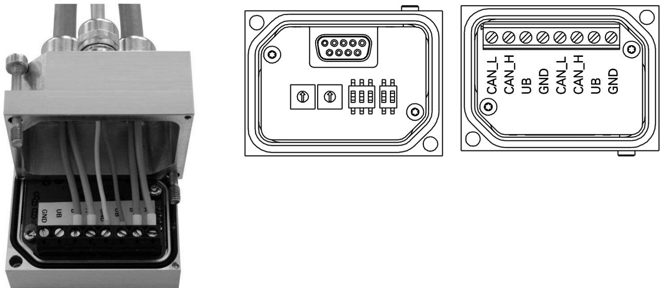
**Note:** Both rotary switches and 3-pole DIP switch are without function.
